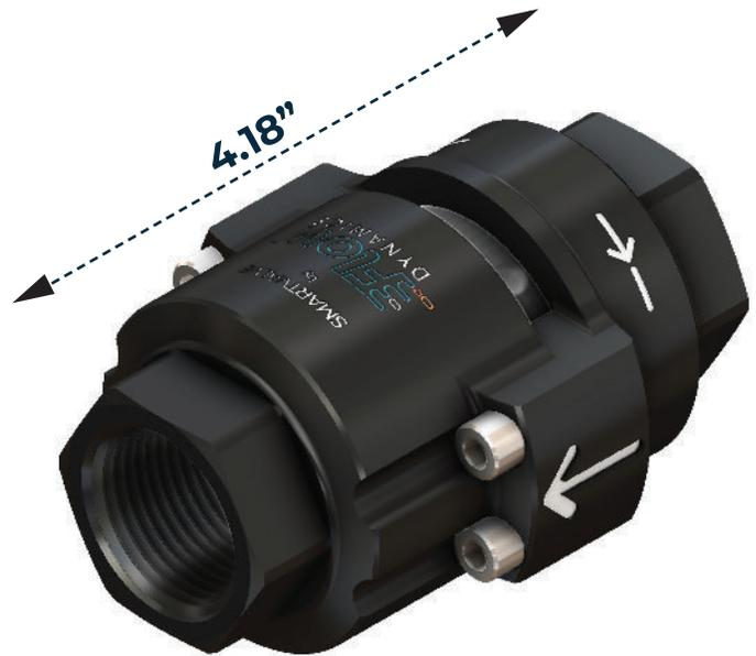
For best results install the Smart Valve downstream of water meter and backflow preventer (if present), but before any other equipment such as a pressure reducer or booster pump. Where possible it is recommended (but not critical) to have 10 diameters of pipe between the water meter and the valve. All flanged installations to use gaskets at each flange.
